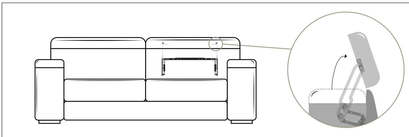
**Benefit:** The STILE hybrid manual headrest is a versatile product, characterized by reduced sizes due to a telescopic adjustment function of the width of the crossbar. 63° rotation, 191 mm lift, 20 mm translation. This headrest guarantees a high comfort level in all its
