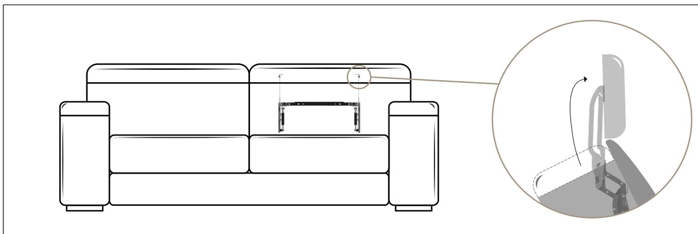
**Benefit:** The STILE extended plus manual headrest is the flagship product of the STILE family. It's one of the most revolutionary and functional products with 102° rotation, 232mm lift and 83mm translation. This headrest
