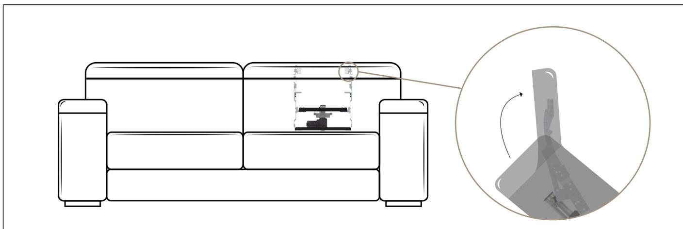
**Benefit:** This motorized headrest is fully upholstered inside the sofa. The very slim structure has the following features: 57° rotation, 54mm shift and 105mm translation. High quality materials and electric kit make this mechanism
