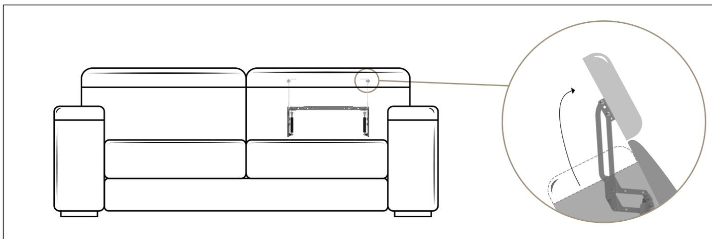
**Benefit:** The manual Stile extended headrest is a versatile product, characterized by reduced sizes due to a telescopic adjustment function of the width of the crossbar (90° rotation, 241 mm lift, 55.7 mm translation). This headrest guarantees a high comfort level in all its
