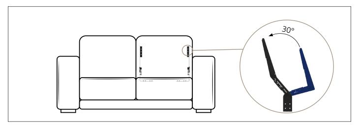
Benefit: The ZED UP manual is a backrest with great potential. It has been designed to be used independently of the measure of the seat; it is mounted on the frame (seat) and is ready for use. It is designed for upholstery with high backrest; 30° rotation when opening, increases the comfort of the finished product. The springs help the user in the closing phase. The easy shape and the formal simplicity make this product highly appreciated.
