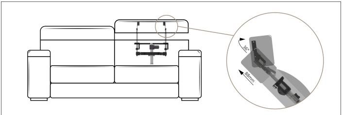
Benefit: VERTICAL spin motorized is an evolution of the VERTICAL motorized headrest. Easy to use, compact and the avant-garde technology makes this product unique. Equipped with a translating movement (88mm) that increases the support
