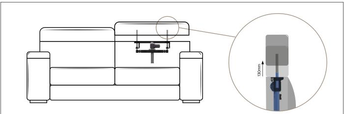
**Benefit:** The **Vertical fly** motorized headrest is a motorized translating mechanism, that allows to adjust the height of the headrest at will. New product of the VERTICAL family, the fly version is lighter and more compact, with an increased translation movement compared to the other products (130mm). Versatile and comfortable, it can be customized with a selection of TEXAS sofa joints, combining the translation with the rotation, enriching the quality of the product.
