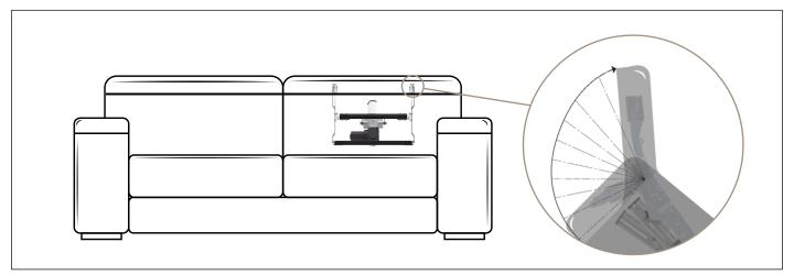
**Benefit:**This motorized headrest is fully upholstered inside the sofa. The very slim structure has the following features: 110° rotation, 179mm shift and 121mm translation. High quality materials and electric kit make this mechanism
