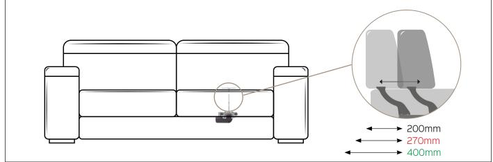
**Benefit:** Motorized backrest support caraterized by high efficiency and quality of the materials and of the electronic components. Its linear movement allows for the backrest to move, differnt configurations 200mm,
