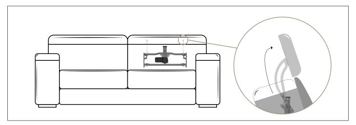
Benefit: This motorized headrest hides itself inside the sofa frame. Highgrade and efficiency materials and electric components. Narrow shape and great versatility (88° rotation, 215 mm rise, 76 mm shift).
