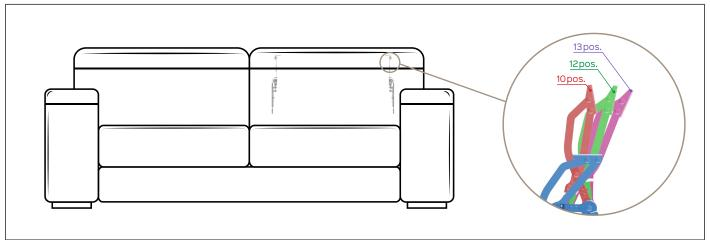
Benefit: The manual NEW CRIPTO headrest thanks to the sequential movement allows the end-user to find the best comfort position. The incorporated parts are in zinc finishing while the visible parts are chromed.
