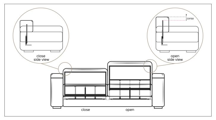
Benefit: EASY BACKREST manual is a back ideal for upholstery with low profile and contemporary design. The use of high quality materials and a durable but light structure, makes this product easy to install and long-lasting. The mechanism moves upwards and is activated by pressing the backrest, flowing up to 112 mm, thus
